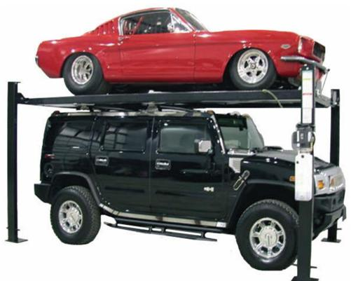
Lifting Capacity 9000 LB Power unit electrical requirement 110 or 220 Volt Shipping weight 1650 lbs. Speed of rise 75 seconds Lifting height in top lock position (height to top of runway) 84" Clearance under lift in top lock position (height to bottom of runway) 81" Length of runway 181"
